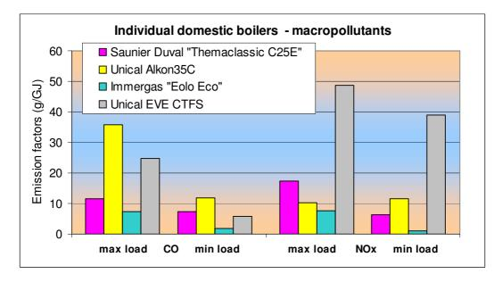
Also the PAH emission factors (following figure) show higher average values in the non-continuous operation mode, while under the same operating conditions the same emission factors are lower for boilers equipped with abatement emission devices, like the pre-mix Immergas boiler and the Unical condensation boiler. The naphthalene is the most significant comparison parameter since the other compounds show negligible values.
