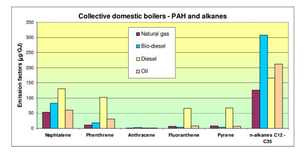
In specific transient operating conditions highest values are found in fuel oil boilers, especially for naphthalene and paraffins. It should be noted as even in biodiesel boilers higher values are found in transient operating conditions.
