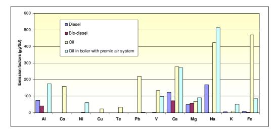
Similarly to the case of the macro-pollutants, even for metals, the biodiesel seems to be the best choice from the environmental point of view. For what concerns the effects of the different technologies, assumed the same fuel, the Hi-Tech fuel oil boilers provide limited iron, vanadium and lead emissions, compared to the conventional technology, although showing a small increase in potassium, sodium and aluminium emissions.
