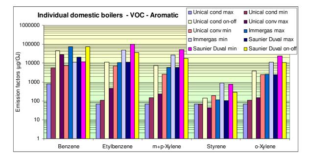
The UNICAL condensation boiler and the IMMERGAS with pre-mix burner, which are the most technologically advanced models, provided the best performances for what concerns the micro-pollutants emissions.
