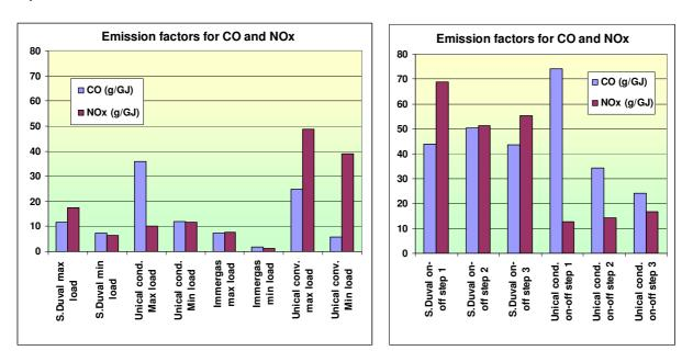
As shown in the figure, the UNICAL condensation boiler and the Immergas with pre-mix burner, which are the most technologically advanced models, provided the best performances also for what concerns the micro-pollutants emissions. The premix burner is efficiently reducing NOx emission also during
