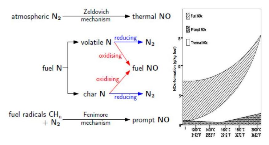
Almost all the NO<sub>x</sub> generated is actually NO (PM 30) and <u>not</u> NO<sub>2</sub> (PM 46), with an overestimation of mass concentration of 50%.
