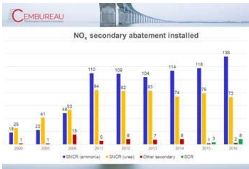
Figure 2: Evolution of plants equipped with SNCR and other techniques in Europe ([12] and CEMBUREAU information)
